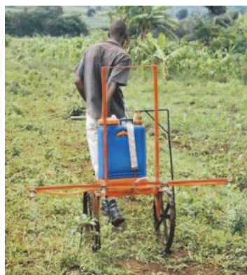
Figure 3. A back-pack sprayer adapted to a towing frame and ground wheel drive to make it into a 4-nozzle, 2 m field sprayer. The operator is distanced from the spray application which reduces the risk of contamination (Photo: Brian Sims).
